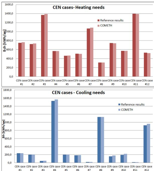
Figure 2: Heating and Cooling needs on all CEN configurations
